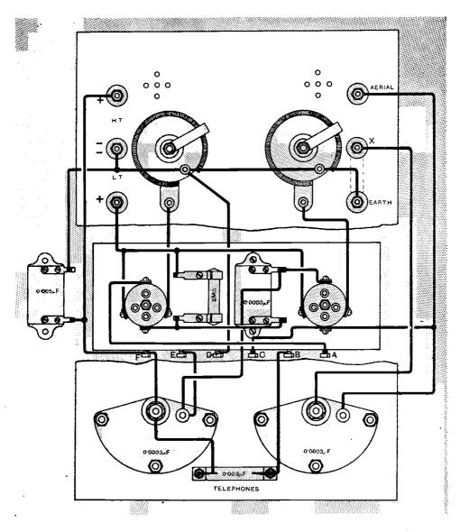
Fig. 4. Arrangement of the components and details of wiring.
