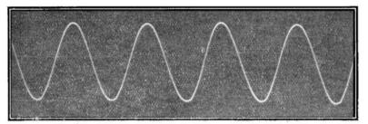
Fig. 11. Photograph of the simple tone from a tuning fork.
