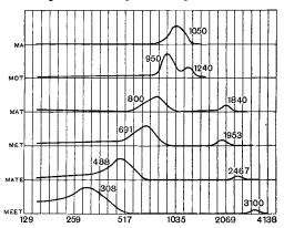
Figs. 17 and 18. Showing the energy distribution at different frequencies for various vowel sounds.
