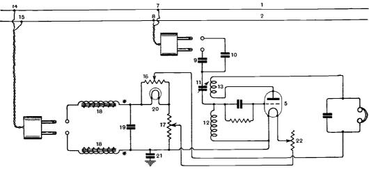
Fig. 2. Arrangement of a receiver which uses the electric lighting wires as the source of power for the anode and filament, and as an aerial.
