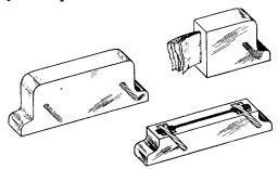
The completed condenser and a sectional vizw showing the appearance of the clamped plates.
