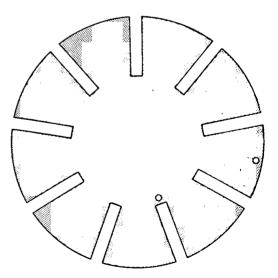
Fig. 5. Card for winding the inductances (exact size).
