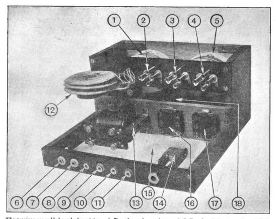
The receiver assembled ready for wiring. 1 Tuned anode condenser, 2 L.F. valve, 3 detector valve, 4 H.F. valve, 5 frame tuning condenser, 6, 7 frame terminals, 8 H.T. -, 9 H.T. +, 10 L.T. -, 11 L.T. +, 12 tuned anode coil, 13 intervalve transformer, 14 telephone jack with break contacts for filament circuit, 15 position for grid leak, 16 primary bridging condenser, 17 grid condenser, 18 H.T. battery bridging condenser.
