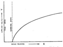
Fig. 7. Relationship between the applied voltage and scale deflection.
