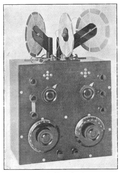
Front view of the two-valve receiver.
