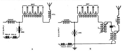
Fig. 1. (A) the original circuit at Leafield; (B) the new coupled circuit.
