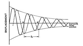
Fig. 6. Showing relationship between displacement and distance from the source of the sound wave.
