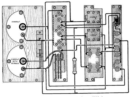
Fig. 6. Diagram of connections showing the actual points between which leads are run.
