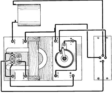
Fig. 4. The internal connections.
