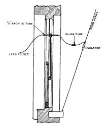
By fixing your lead-in in this way opening and closing the window is not interfered with.
