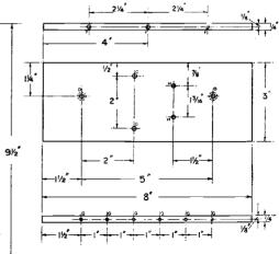
Fig. 2. Drilling diagram for the panels. The size of drills should be as follows :—A 7/16", B 5/16", C 5/32", and countersunk for No. 4 P.A. screws; D 5/32", L 5/32"; F 4 B.A. screw thread.
