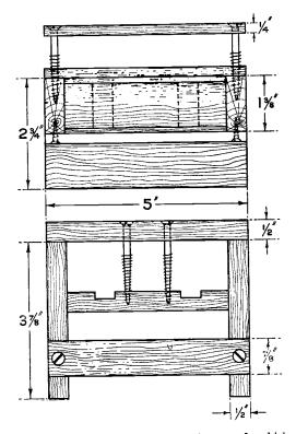
Fig. 3. Details of the wooden framework which carries the Weston relay, grid battery and value platform.
