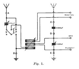
Referring to Fig. 1, it will be seen that the receiver will be inductively coupled to the aerial when the aerial and earth wires are connected to terminals A and B respectively. A directly coupled circuit will be provided when the earth is connected
