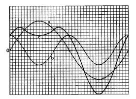
Fig. 10. Another example where the octave b has started before the fundamental a.
