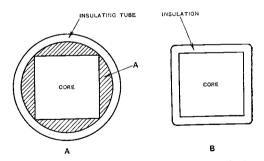
Fig. 1. In sketch A, a circular former which just fits over the core is employed; hence, the space marked A is wasted. In sketch B, the coil is wound on a rectangular former.
