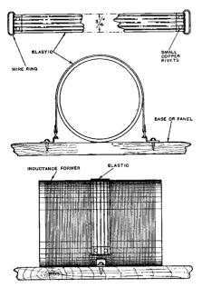
Coil fixing with elastic band.
