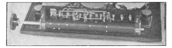
One of the most efficient methods for changing out valve circuits, when switching H.F. and L.F. amplifiers in and out of action, is by means of a barrel switch. The switch shown here is of simple design and is attached immediately beneath the valve platform so that many of the spring contacts are actually carried by the valve stems. The switch, which has been designed by Mr. E. J. Baty, B.Sc., is here shown fitted to a Baty receiver.
