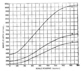
Fig. 1. Tuning curves of the Acme Variometer.
