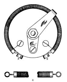
insulated covering. A suitable winding is No. 36 Eureka wire.
