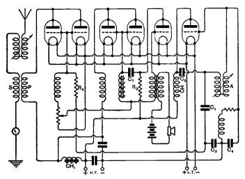
Fig. 1. Connections of the wireless telephone transmitter. It will be seen that a master oscillator is employed to excite the grids of two power valves connected in parallel. The modulator comprises two valves in parallel, and a speech amplifier.
