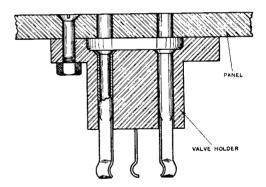
Fig. 5. Sketch of a valve-holder which is designed to be fitted below the panel.
