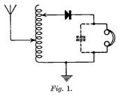
For the range of wavelengths between 300 and 500 metres, the tuning coil may consist of 150 turns of No. 20 enamelled copper wire on a cylindrical former 4 inches in diameter. A condenser may be connected across the telephones if an improvement is thereby obtained in the quality of reception.
