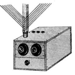
Fig. 7. The containing cabinet with lower portion for accommodating the H.T. and L.T. batteries. The stem of the frame aerial passes clear through the wiring of the instrument, and the weight of the batteries makes a suitable base for giving vertical support to the frame.
