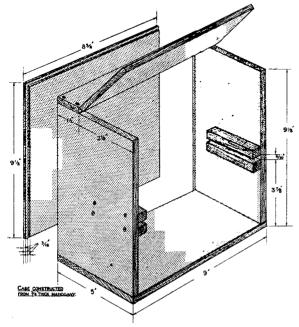
Fig. 3. Dimensions of the case containing the receiver.
