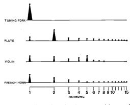
Fig. 14. Illustrating the frequency richness of various instruments.
