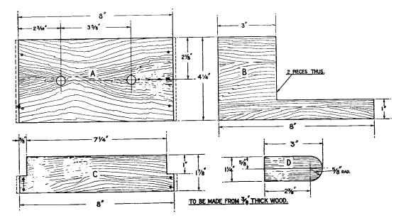
Fig. 2. Details for constructing the wooden pieces.
