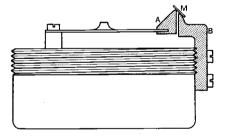
Fig. 8. A simple arrangement for showing telephone diaphragm vibrations.
