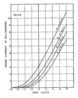
The valve takes a filament current of 0.22 ampere at 5 volts, which is similar to that taken by the D.E. 5 valve.
