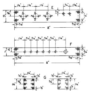
Fig. 3. The ebonite pieces, for valve holder platform, terminal strip and condensers. Size of holes; K <sup>3</sup>/<sub>8</sub>", L 7/32", M 5/32", N <sup>1</sup>/<sub>8</sub>" countersunk on top side for No. 4 wood screws, P <sup>1</sup>/<sub>8</sub>" countersunk for No. 4 wood screws, Q <sup>1</sup>/<sub>8</sub>".
