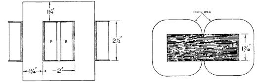
Fig. 3. Scale drawing of the transformer.
