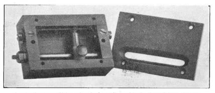
A potentiometer utilising a length of pencil graphite for the resistance element.
