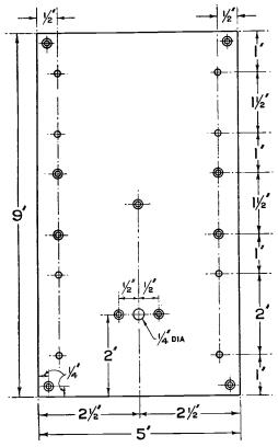
Fig. 1. Details for setting out the top panel.
