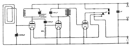
Fig. 1. Circuit of frame aerial receiver, with tuned anode high frequency amplifier, valve detector, and note magnifier. Reaction coupling is unnecessary owing to the low degree of damping possessed by the frame aerial.
