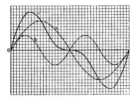
Fig. 9. Resulting tone c formed of sine wave a and its octave b,
