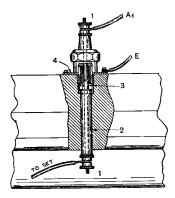
Fig. 1. A lead-in tube.
