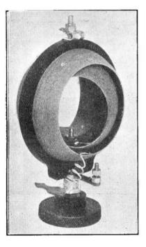
Hence in well-designed variometers we find the windings are separated by a distance which is considerably more than is required from a mechanical point of view. It is well known that the effective resistance of a coil may be reduced by the employment of a large gauge of wire, and by reducing the amount of material in the supports of the coils to a minimum. A variometer which appears to have desirable electrical properties is shown in the accompanying illustration. It will be
