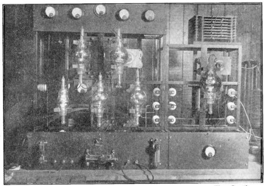
[Photo : Barratt's. The Edinburgh Relay Broadcasting Station 2 EH, is now giving great satisfaction. The photograph provides a clear view of the transmitting panel.
