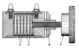
The "Oojah" rheostat. A is the knob, B the fixing nut, C the discs of copper foil, and D the resistance elements (graphite).
