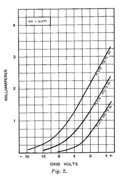
The valve has a magnification factor of about 5, and an impedance of from 35,000 to 20,000 ohms according to the plate potential used; see Fig. 3.
