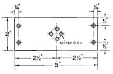
Fig. 5. The valve platform.
