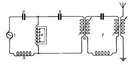
Fig. 2 Showing the use of a tuned circuit to reduce the strength of harmonics generated by the machine generator.
