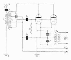
Fig. 6. Final type of oscillation circuit.
