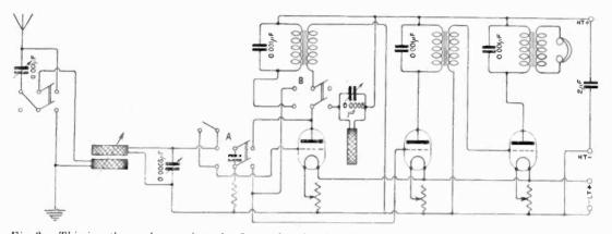
Fig. 3. This is a three-value receiver the first value of which may be used as a H.F. amplifying value or as a detector value.
