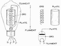
Fig. 10. Component parts of the valve and the method of representing them in wireless circuits.
