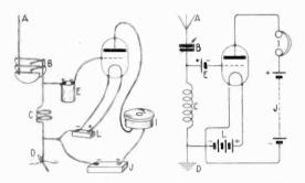
Fig. 11. Pictorial and diagrammatic representation of a valve circuit.
