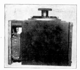
The Buzzer Wavemeter.
