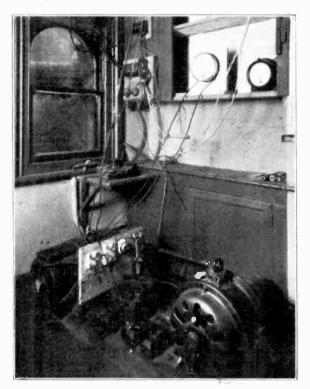
Fig. 2. The generator unit with driving motor.
