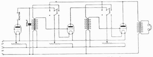
Fig. 1. The circuit shows the switching of two note magnifying values.
