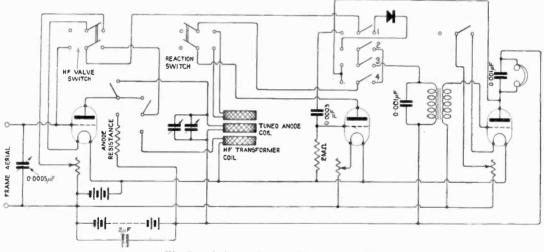
Fig. 2. A three-value experimental receiver.
