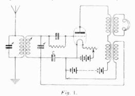
transformer in the anode circuit which passes the low frequency impulses through the valve after being rectified. The condenser "C" is required to pass the high frequency current from the secondary tuned circuit to the valve which is acting as a rectifier, and also a low frequency amplifier.
