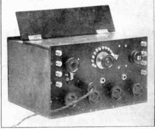
combination of valves to another. If the photographs and diagrams are examined, it will be seen that there are three plug sockets and three switches on the front of the instrument. The switch on the right is a miniature tumbler switch made of ebonite, serving to switch all of the valves on and off as required. This is an advantage
