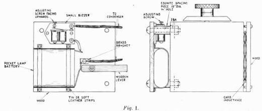
Method of assembling buzzer and battery.
