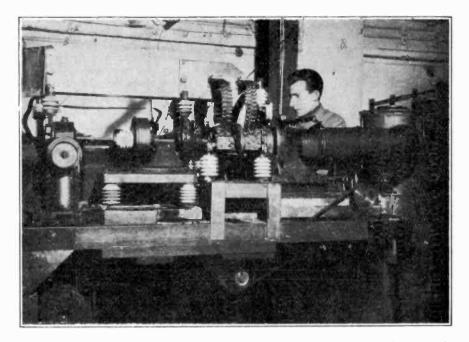
Fig. 3. The spark gap, with ventilated revolving electrodes, and  $\operatorname{arranged}$  so that the total sparking distance is synchronously broken down by the discharge a condenser bank separate from the main oscillator.
