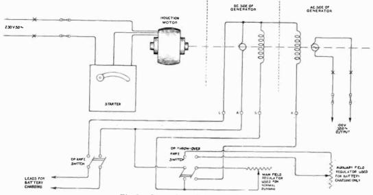
Fig. 3. Connections of generator unit.
