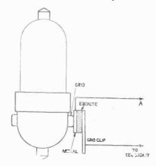
Fig. 11(a). A method of tapping-in on to the grid circuits to vary the number of values used.
