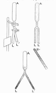
Fig. 6. Experiments with an electroscope. The uneven distribution of the electrons constitutes an electric charge.
