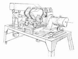
Fig. 2. The spark discharger, showing the two gaps.
