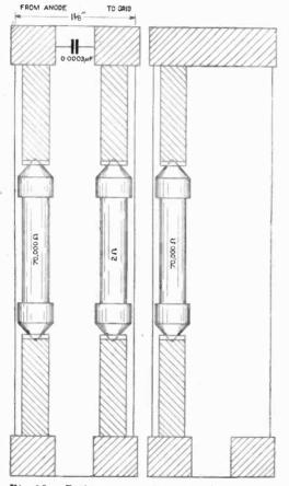
Fig. 10. Resistance-capacity units to replace transformers on longer wavelengths.
