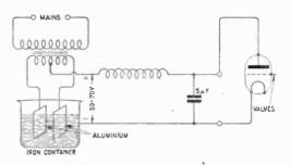
Fig. 1. The Electrolytic Rectifier and smoothing circuit.
