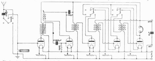
Fig. 1. A 5-valve receiver with 1 H.F., 1 Detector, and 3 L.F. valves. The H.F. valve is transformer coupled and the reaction coil is coupled with this transformer. Switches are provided for culting out L.F. valves.
