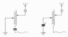
Fig. 7. An earth connection may be combined with the counterpoise in the manner indicated in the figure. The correct connection to be employed depends essentially upon the transmitter connections, and the experimenter will have no difficulty in adapting the arrangement to meet his own needs.
