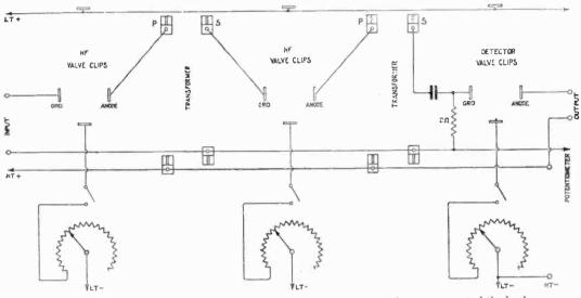
Wiring lay-out of the H.F. Amplifier showing the special arrangement of the leads. Fig. 9.
