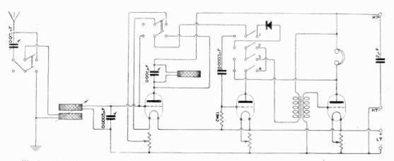
Fig. 2. A 3-valve receiver. A crystal detector may be used instead of the detector valve when required.
