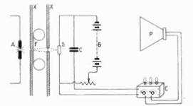
Fig. 14. Circuit arrangement of Ruhmer's photographophone.
