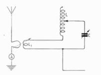
Fig. 3. The coil L and variable condenser C form part of the oscillating circuit LC of Fig. 1. The remainder of the circuit not shown is the same as Fig. 1, but here the aerial circuit includes a hot-wire anneler and a single turn.
