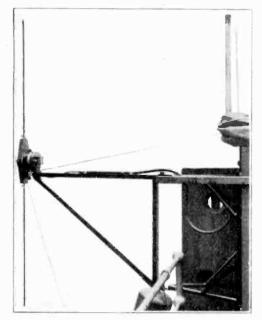
Marconi Wireless Beam Receiving Antenna on Ship's Bridge,
