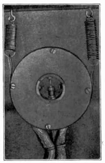
Photo—Courtesy. Westinghouse Electric Co. A suspended glow discharge microphone.
