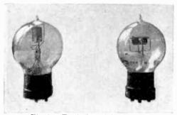
Fig. 9. Typical receiving valves.
