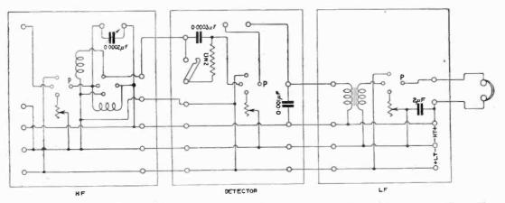
Fig. 2. The diagram shows a H.F. panel coupled to a detector panel and followed by a note magnifier. The windings shown in the first panel are those of a H.F. transformer.
