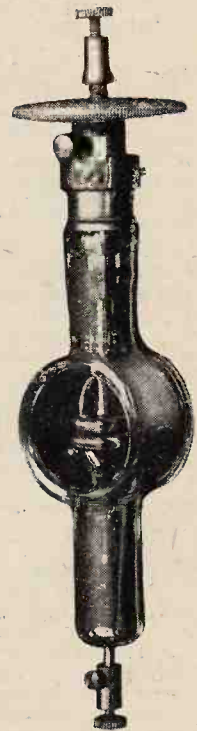
The "Kerr" cell shown by Messrs. Isenthal and Co., Ltd. This device is complementary to the ordinary photo-electric cell, its use being to reconvert electric impulses into variations of light density.
