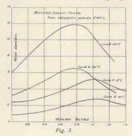
500 per sec. Readings were taken of Ir at various mechanical pressures for various temperatures, from 16° C. to 550° C. for different grs. load on the crystal.
