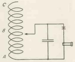
A-C at B, or by providing separate sections of inductance which can be added or taken away as required.
