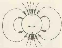
Fig. 6.—Section of earth's magnetic field shewing paths of election through the outer atmosphere.
