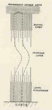
Fig. 8.—The effect of the diurnal layer on shape of wave.
