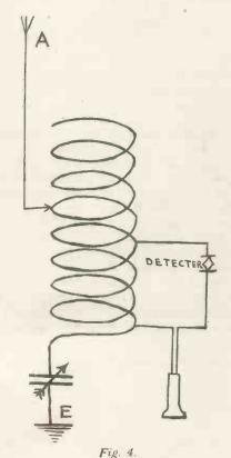
former on which the coil is wound be in the form of a tube, then any conducting material which may be present on the inner wall of the tube will form a condenser with the wire on the outer wall.
