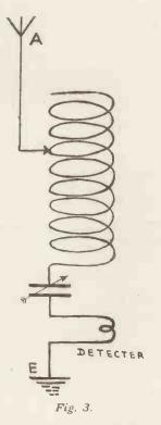
inductance be shunted by a condenser, then longer waves can be tuned to than by the inductance alone.
