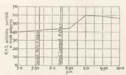
Fig. 4.—Paris Sunset Test, July 26, 1913: Paris Antenna Current, 43-45 amperes. Weather clear.
