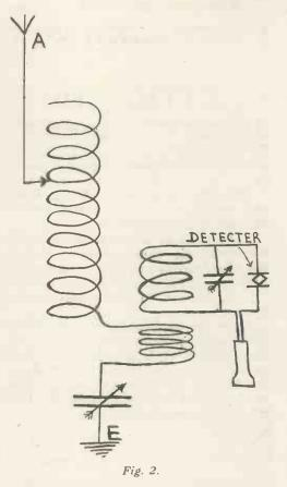
Another point to be noted is that no part of the coil should be short-circuited, whether it is in circuit or idle. The short-circuited coil will absorb energy from the rest of the circuit, and the effect is greatest when the ratio of short-circuited coil to the part in use is large—e.g., when only one or two turns are short-circuited.
