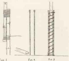
bindings will probably need plugging with pieces of wood. If plugs are used, they should be driven in bindings in a downward direction to prevent them from working out should bindings stretch in very dry weather.
