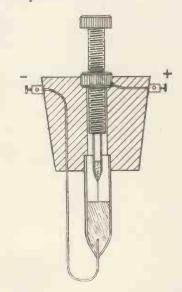
The positive electrode is put into a glass tube of a little larger diameter, which contains some sulphuric acid (10 per cent. solution) and the negative electrode of lead.
