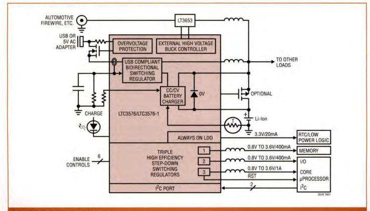
Figure 1: LTC3576 simplified block diagram
