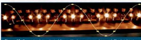
Figure 13: Open circuit terminated line, with sinewave superimposed. The brightest lamps are now at the line ends compared with Figure 12
