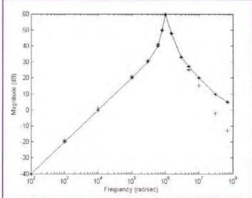
Figure 3: Experimental (+) and calculated (\*) results obtained from the bandpass realisation
