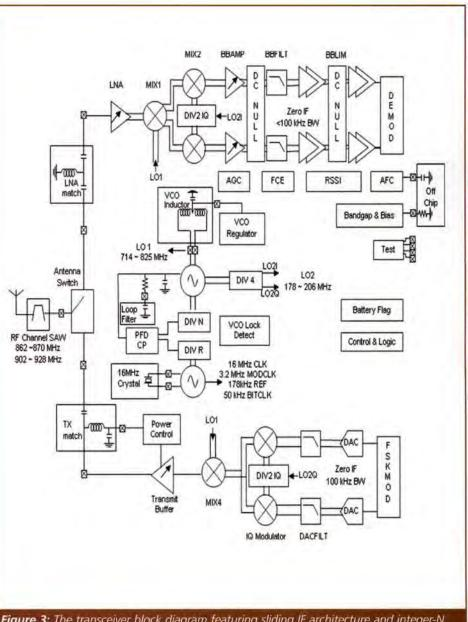
Figure 3: The transceiver block diagram featuring sliding IF architecture and integer-N synthesiser
