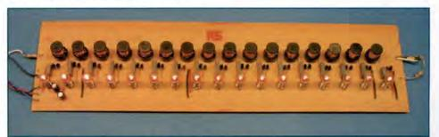
**Figure 11:** Board layout on the left are a white and black pair of wires which connect to a power amplifier, through the matching resistor, and a black, red and blue triplet connected to the +/- 12V supplies, with blacks being commoned. On the right is the load resistor clipped to the output
