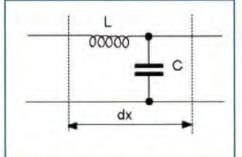
Figure 3: Lumped constant with single inductive and capacitive element for a line section dx; assuming that the leakage and series resistances can be ignored
