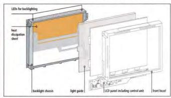
Sharp has launched an enhanced range of LED backlit liquidcrystal panels for industry applications. The portfolio now incorporates five displays in the screen diagonals of 3.5 to 15 inches.
