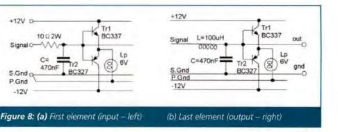
along the line, and have sufficient elements to demonstrate peaks and troughs, the number of elements needs to be divisible by a multiple of two so that half and quarter wavelengths can be illustrated. Choosing 16 elements requires each element to have a time delay of  $6.25 \mu s$ . This sets one of the two characteristics of the model line.
