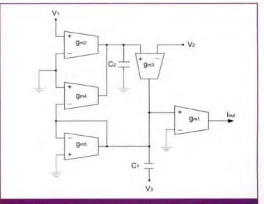
Figure 1: Proposed universal filter circuit with input voltage and output current
