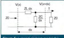
Figure 6: Lumped element model this time showing voltage and currents in line
