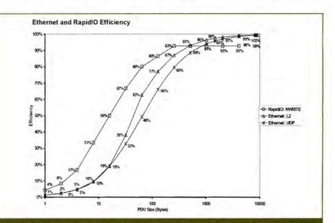
**Figure 1:** Ethernet achieves its best efficiency with a maximum payload, although this comes at the cost of increased latency jitter. By balancing large payload jitter against small payload inefficiency, an alternative interconnect standard like RapidIO technology achieves better overall efficiency across the payload sizes most common to embedded backplane applications
