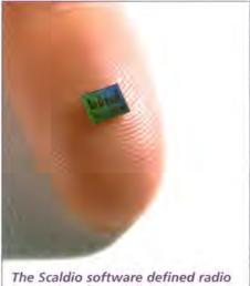
The Scaldio software defined radio transceiver from IMEC
