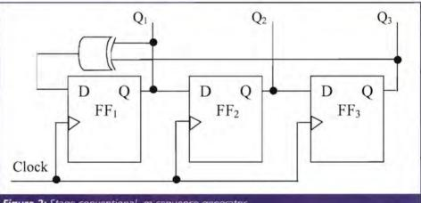
Figure 2: Stage conventional m-sequence generator
