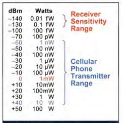
Figure 1: dBm values and their corresponding values in Watts
