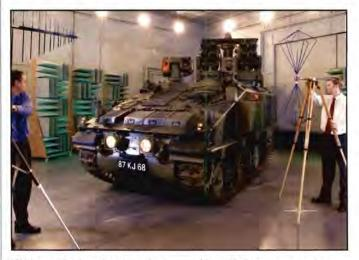
UK-based test and certification company TRL Compliance has opened a new 18x14x6m EMC test facility in Malvern, the UK. This is a large size chamber, which could easily accommodate large military, agricultural and industrial vehicles and equipment.
