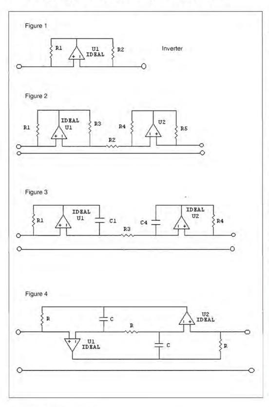
The end circuit represents a floating negative inductor using only two op-amps. It obviates use of GIC (General Impedance Converter) that requires more than four opamps for the same purpose. It requires two matched capacitors and three matched resistors.
