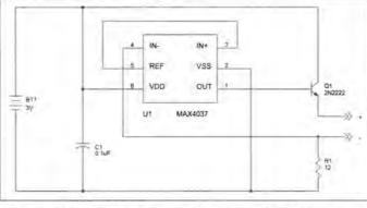
tional amplifier with a built-in 1.232V reference. The positive input of the op-amp is connected to the reference directly. The negative input is through a  $12\Omega$  resistor to ground. Output of the op-amp drives an NPN transistor to increase the driving current. Terminals '+' and '-' are used to probe the PCB shortage. A digital voltmeter (DVM) in the mV range is connected to these two terminals to get the milliohm reading.
