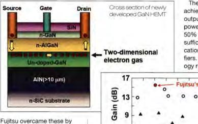
The characteristics achieved, including maximum output of 101W, maximum power-added efficiency of 50% and gain of 15.5dB, are sufficient for practical application of GaN HEMT amplifiers. In addition, the technology reduces GaN HEMT
