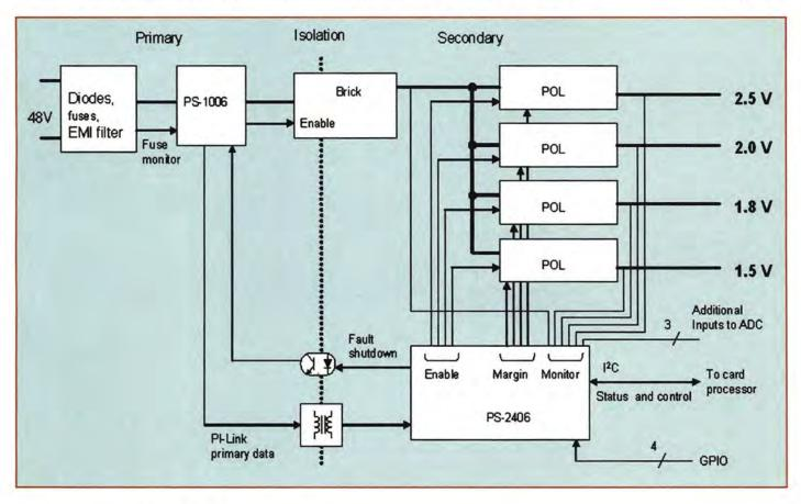
Figure 6: Communication link components condition, it turns off the MOSFET used for inrush current limiting. A time delay is included to prevent nuisance tripping.
