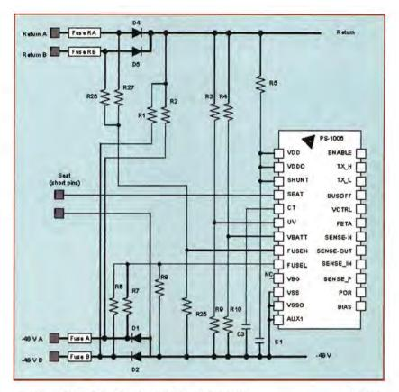
management function to include the primary side. Because of the high voltages and isolation requirements, the PS-1006 uses mainly analogue inputs and operating parameters are set by external resistor values.
