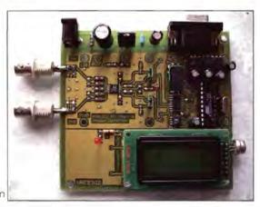
Figure 10b: VRC8302 prototype measurement system
