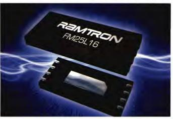
lead-free 8-pin SOIC package.
