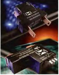
voltage to maintain the 'on' state. The KG100 has a SPST contact arrangement and an operating time of 20mS, the K200 has DPST contacts with an operating time of 30mS. All units are available with operating coils of 12, 24, and 48V, however the K100 is also available with a 6V coil. The relays can operate in a temperature range of -40°C to +70°C. The relay has a 60A motor load rating from UL that requires a minimum of 50 switching cycles at 600A. www.switchtec.co.uk
