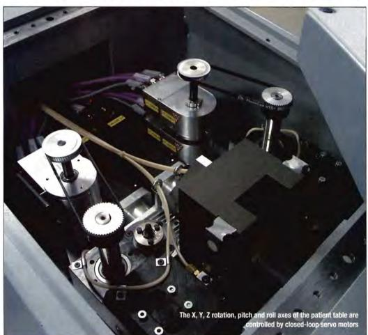
A new high-integrity motion control system used in proton beam irradiation therapy for treating tumour patients is one of the first such machines to be based on the Linux operating system (OS). IPG of Switzerland designed the novel eight-axis control system for the machine, based on components from Baldor and the Mint-language motion commands, specially ported to run under Linux for this project.
