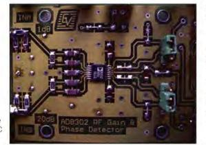
Figure 10a: The gain and phase detector IC AD8302
