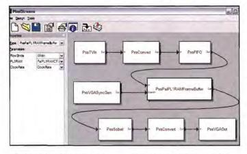
abstraction. In addition, Pixel-Streams includes an IP reuse graphical editor as an entry tool for imaging algorithms to provide ease-of-use and design productivity in a familiar blockbased methodology.
