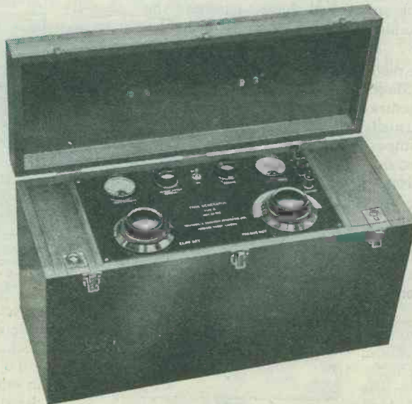
CONSTANT-OUTPUT TONE GENERATOR A constant-output tone generator. This instrument is made by Technical and Research Processes, Ltd., of which Capt. H. J. Round is the head
