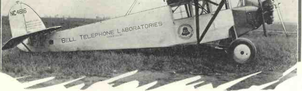
The rod aerial and wind-driven generator can be seen in this photograph of the Laboratories' plane
