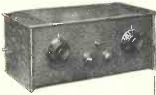
The new Cossor Empire screened-grid three-valve kit set which is certain to be very popular. (Stand 52)
