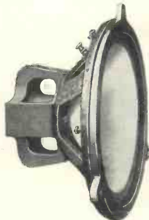
An interesting Epoch permanent magnet moving-coil loud-speaker. No tools, except a screwdriver, are required for its assembly
