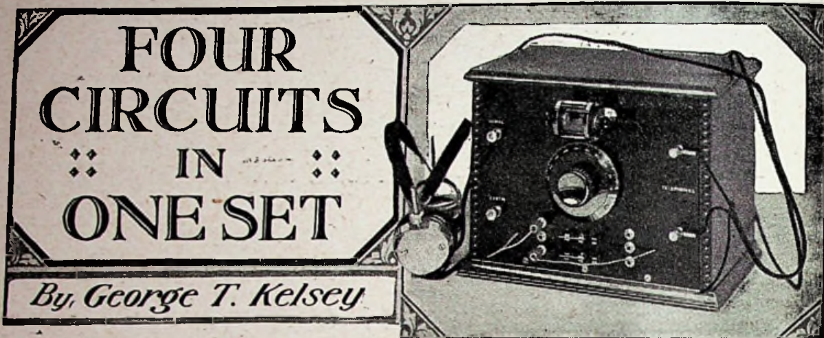
A novel crystal receiver giving a circuit for every need
