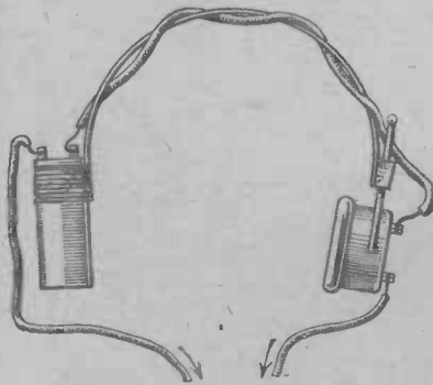
Fig. 1.—The testing instrument is made from a pair of telephones and a battery.
