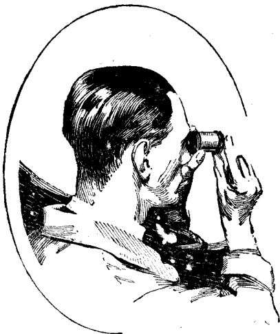
Illustration showing laboratory worker taking a temperature reading by means of the Pyrometer.
