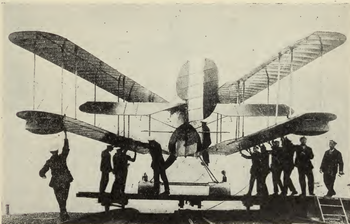
A seaplane which folds its wings while ashore
