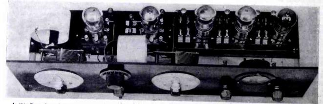
In this illustration only two or three connecting wires are visible. All leads carrying radio-frequency currents are run above the sub-panel and all A and B battery leads are run beneath
