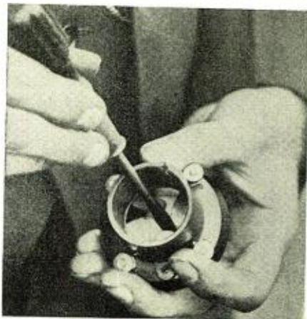
By means of a screw driver, bend up the socket contacts to make good contact with the tube
