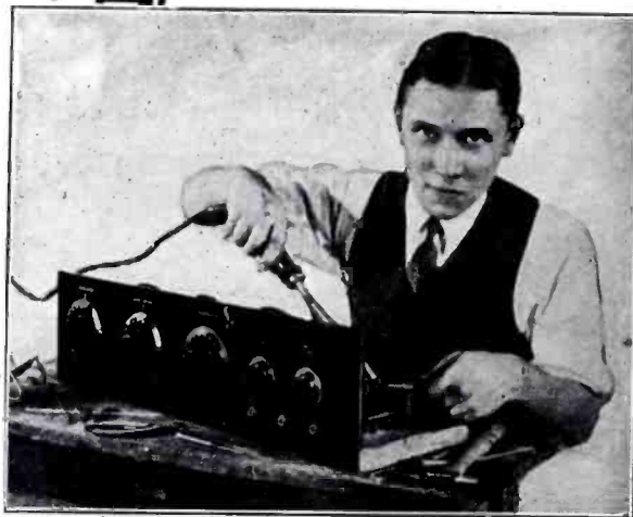
Front View KD-50 Neutrodyne Being Assembled
