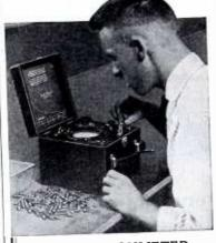
THE MEGOHMETER Designed by engineers to test "PRE-CISION" RESISTANCES. Accurately measures any resistance between .02 megohms (20,000 ohms and 12 megohms (12,000,000 ohms).
