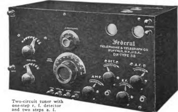
antennas but also on indoor loops. Three rheostats are provided to control the tube filaments and there is also an amplification control.
