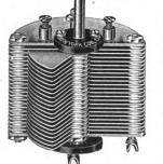
New York Coil Company's Vari-able Condensers have set a stand-ard by which all others are judged. Plates are of extra heavy aluminum, accurately spaced. The framework of the supporting elements is such that permanency results. Adjust-able bearings with provision to take up wear and means for always in-suring positive contact is provided.
