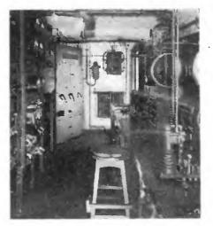
This is the radio room of the S. S. Kamoi, fuel ship of the Japanese Navy. The ship has what has been termed the "most elaborate radio equipment of any ship afloat." There are three transmitters and three receivers
