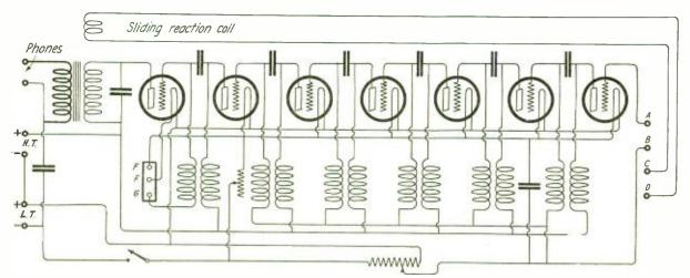
Fig. 5. Seven-tube amplifier especially suited for long-wave trans-Atlantic reception
