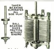
The tension as well as adjusting is accomplished by tightening end thrust plug, causing a thrust between a hardened steel ball and a 45 degree tapered brass bushing, this insures smooth running and a contact equal to a soldered joint also a take-up for wear in years to come.
