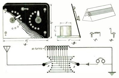
Simple and ingenious crystal tuner and detector with triangular cage-type antenna strung inside the gable roof of the house
