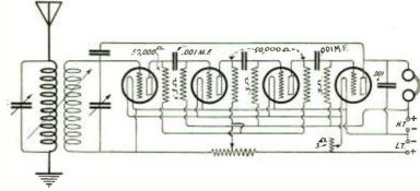
Figure 7. Resistance-capacity coupled amplifier system
