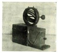
Figure 3. Home-made variometer and variable condenser
