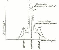
Figure 9-Distortion of modulated wave due to low receiver decrement
