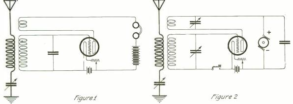
Circuit diagrams showing similarity between regenerative receiver and CW transmitter
