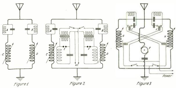
Wiring diagram of the system of duplex transmission on a single aerial and ground
