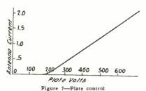
For plate voltages exceeding 200, we see this curve is a straight line, and therefore if the plate voltage is not reduced below 200, good quality should result when using this method of modulation.
