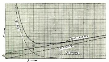
Figure 2. Component curves in measuring antenna resistance
