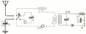
Figure 1. Diagram for testing antenna resistance
