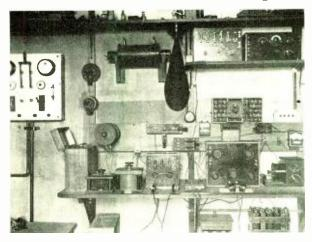
F. Leverrier's station, Sydney, Australia, equipped with resistance-coupled frequency amplifiers
