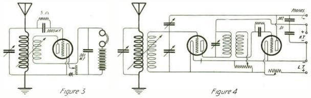
One and two tube English receivers, the latter using a tuned transformer
