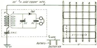
How the antenna was stretched over the rafters
