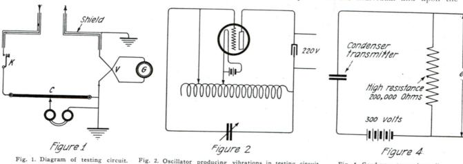
Fig. 2. Oscillator producing vibrations in testing circuit.
