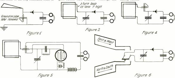
Figure 1. First antenna in 25-foot hallway. Figure 2. Modification into a loop. Figure 4. Addition of variometer for tuning. Figure 5. Ease of converting to a bulb set. Figure 6. Use of two fixed directional antennas
