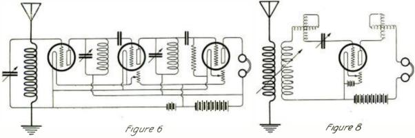
Tuned anode circuit and an effective single-tube short-wave receiver
