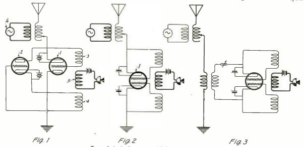
Types of circuits for power modulation in radio telephony
