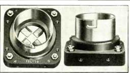
Our No. 666 positive contact socket has brass receptacle, nickel plated, moulded into bakelite socket. Allowance made in diameter of receptacle for the varying diameters of tube bases. Socket contacts insure certain and positive contact with the end and side of prongs of bulb. As socket is moved in the notch a pressure is immediately exerted on the side of the phosphor bronze contacts.
