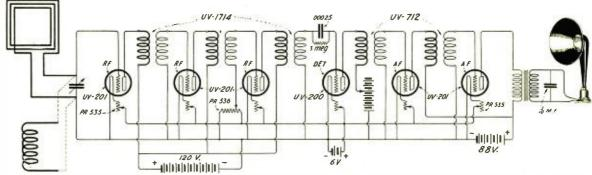
Figure 1-Hook-up of the R.F.-A.F. amplifier
