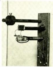
l-Meter transmitter used in the demonstration of directional radio. Transmitters of several hundred watts have been successfully used in tests of directional radio by reflectors on wavelengths between 1 and 15 meters
