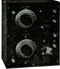
Regenerates wave lengths of (80 to 825 meters perfectly
