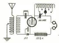
Ans. 1. Suggest that you employ the tuned plate circuit as shown. Wind a tube 10 inches in length by 3 inches wide with about eight inches of No. 24 D.C.C. taking a tap off every inch. Connect as shown.
