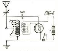
The hook-up used in the short-wave receiver at Oahu, H. T., for reception of Pacific Coast amateur signals
