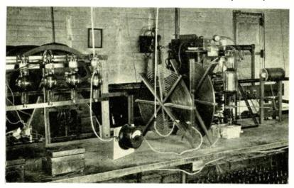
Transmitting equipment of WGY station. The large oscillator tube is shown at the right and the modulator tubes at the left, with meters, coupling inductances and filter condensers
