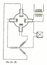
The rectifier for three-phase current
