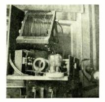
Self-rectification 10-watt C.W. set of 2OM station which has covered remarkable distances considering the receiver used
