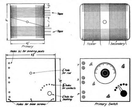
Figure 1-Constructional details of the vario-coupler
