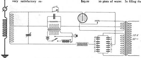
Figure 1-Circuit diagram of the 5-watt vacuum tube transmitter
