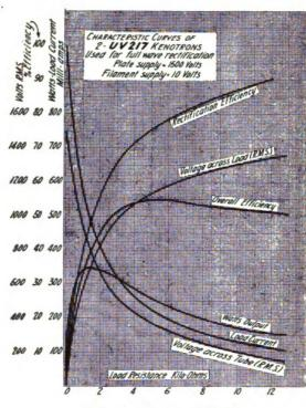
Figure 18-Load characteristics
