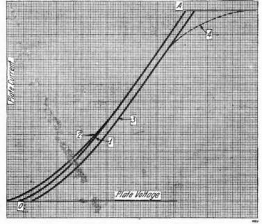
Figure 9-Modifying factors of the characteristic curve
