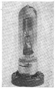
Figure 2-UV-217 Kenotron mounted in socket
