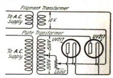
Figure 17-Circuit for full wave rectification
