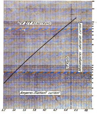
Figure 5-Saturation current graph
