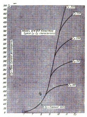
e 7—Volt ampere characteristics showing effect of space charge in limiting the electron current Figure
