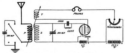
Figure 2-Hook-up for best results of vario-coupler
