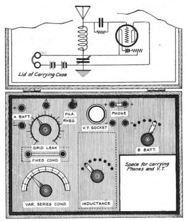
The portable radio set assembled
