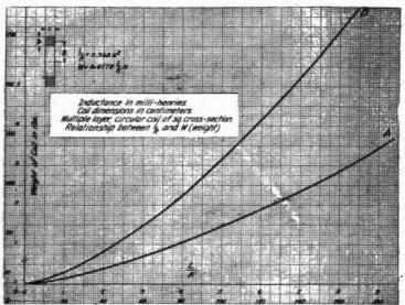
Figure 4-Graph for weight of coil in lbs.
