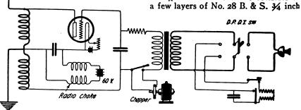
Figure 2-Hook-up for the transmitting set
