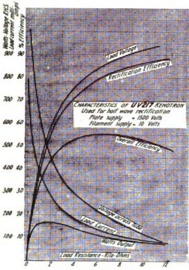
Figure 12-Load characteristics
