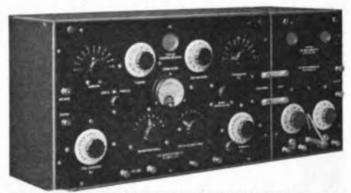
KENNEDY TYPE 110 UNIVERSAL REGENERATIVE RECEIVER WITH TYPE 525 TWO-STAGE AMPLIFIER
