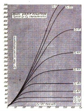
Volt ampere characteristics showing limitation of current due to temperature
