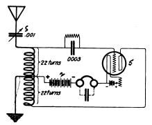
Figure 1—Receiving circuit that simplifies tuning
