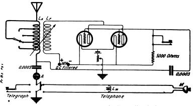
Figure 1-The complete transmitting circuit excluding the filter
