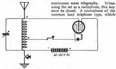
Figure 1—Circuit diagram of a simple CW transmitter
