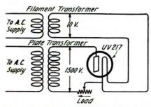
Figure 16-Circuit for half-wave rectification
