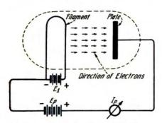
4—Circuit to determine relation ween filament and plate currents
