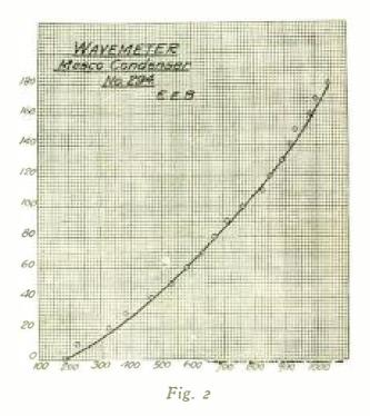
be located where loud signals are obtained in the head telephones. This indicates that the circuits of the wavemeter are in resonance with the antenna system and by reference to the table of wave-lengths corresponding to the degrees on the variable condenser the required reading is quickly obtained.
