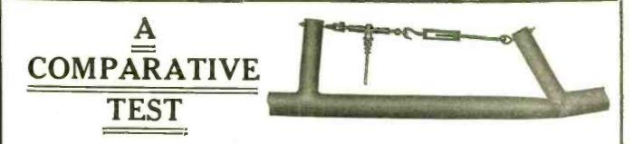
This cut, reproduced from a photograph of a test made to demonstrate the superiority of the Interlock Weld (the branch on the left) over the ordinary butt weld (the branch on the right), speaks for itself.
