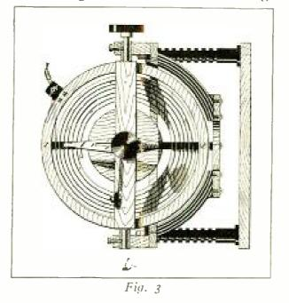
Detail No. 1 is the wood back or base piece which should be of 3⁄4 of an inch stock and perfectly true as this is the foundation for the entire instrument Holes are drilled in the corners, as shown, for 3⁄8 of an inch flat head brass machine screws to mount the columns. Detail No. 2 is the top panel which is mounted on top of the columns and supports the primary helix. The large circular opening shown is bevelled to agree with the helix supporting pieces,
