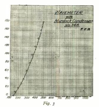
becomes an exceedingly useful piece of apparatus for the calibration and sensitive adjustment of receiving tuners. It may also be used to calibrate coils of wire to a definite range of wave-length, thereby removing all doubt in the experimenter's mind concerning the dimensions of a coil for a given purpose.
