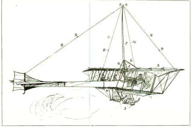
Fig. 11.—In this application of wireless to aeroplanes, the inventor consolidates one element of the antenna structure with the aeroplane structure, and forms the second by the use of an insulating mast and conductors
