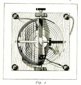
corrugated, hard rubber posts. On these posts is mounted a second wood panel having a circular opening therein and supporting four hard rubber, arcshaped pieces which serve to mount the primary helix. Adjustment of the number of active turns is made by the usual contact clips, of which, in this case, there are two, one being shown in Fig. 1.
