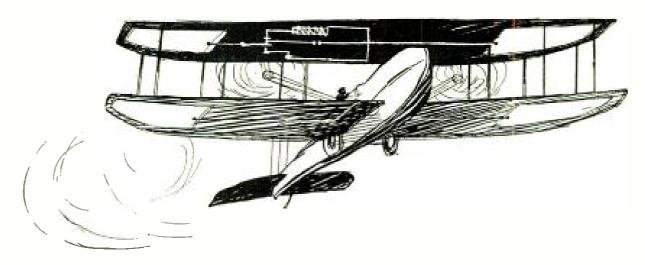
Fig. 10.—Wireless-equipped aeroplane without antenna. The inventor has substituted two extended surfaces of conducting material, so as to form the two capacities of a horizontal antenna. From these surfaces, made of aluminum foil, conductors are run to the signaling instruments
