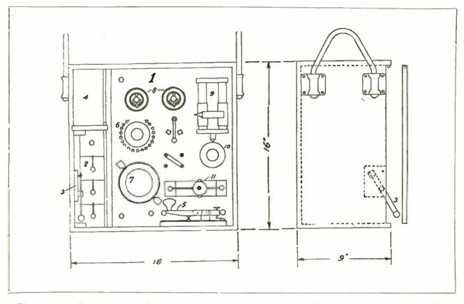
Fig. 3.—(1) Receiver, (2) Batteries, (3) Battery cutout, (4) Telephones, (5) Manipulating key, (6) Aerial tuning inductance, (7) Aerial tuning condenser, (8) Crystal holders.
