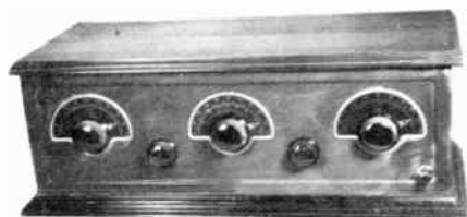
STEWART WARNER MODEL 300 5 TUBE T.R.F. 1925 $75.00
