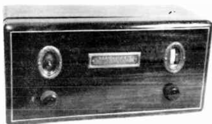
RADIOLA 16 AR-924 6 TUBE RECEIVER UX 20iAs 1927
