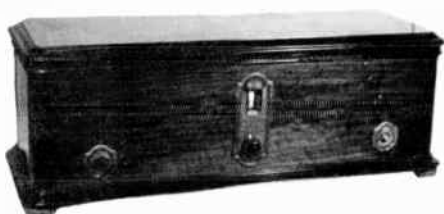
RADIOLA 17 AR-927 ONE OF THE FIRST AC RECEIVERS 1928
