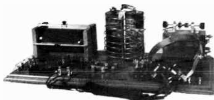
TRANSMITTER-RECEIVER USING CARBON DETECTOR 1917
