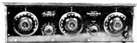
RADIODYNE 6 TUBE T.R.F. USING 199 TUBES 1924 S.P. $150.00 WESTERN COIL CO.
