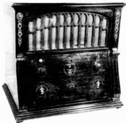
RADIOLA X REGENOFLEX 4 WD 11 TUBES 1925 S.P. $245.00
