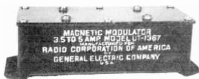
RCA MAGNETIC MODULATOR USED IN ANT. CIRCUIT 1922
