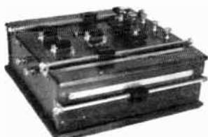
MARCONI TYPE D TUNER AMERICAN MARCONI CO. ALSO MADE BY UNITED WIRELESS. 1905
