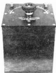
WIRELESS SPEC. CO. .003 IP-301 VAR. CONDENSOR 1919
