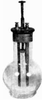
BICHROMATE BATTERY PLUNGER TYPE ABOUT 1900
