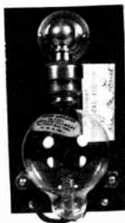
DE FOREST SPHERICAL AUDION DOUBLE GRID & PLATE 1909
