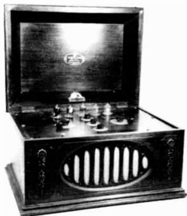
RADIOLA VIIIB & IX 2 CIRCUIT TUNER 5 TUBE DET. AMP. AR-907 1923 S.P. $245.00
