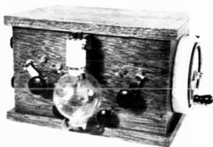
DEFOREST AUDION DETECTOR TYPE RJ4 1909 $18.00 COMPLETE
