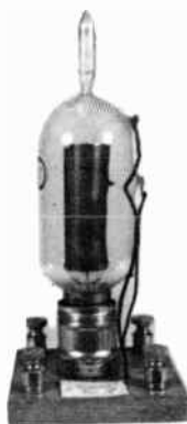
MARCONI TUBE MADE BY H. J. ROUND 1911
