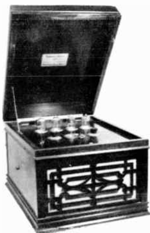
RADIOLA GRAND 4 WD 11 TUBES REGEN. RECEIVER 1922 S.P. $150.00
