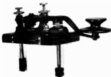
WIRELESS SPEC. APPARATUS 50 AMP KEY ABOUT 1917
