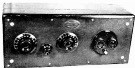
ATWATER KENT MODEL 20 5 TUBE T.R.F. 1924 $80.00
