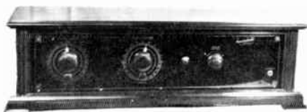
PREMIER RADIO MODEL 7A 5 TUBE REFLEX 3 STAGES OF R.F. CRYSTAL DETECTOR 3 STAGES AUDIO 1924 $250.00
