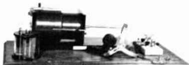
CLAPP-EASTHAM LONG WAVE RECEIVER 1914 FERRON DETECTOR
