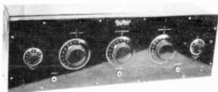
FREED-EISMANN NR-7 6 TUBE NEUTRODYNE 1924 $150.00
