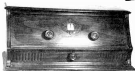
GILFILLAN MODEL 10 5 TUBE NEUTRODYNE 1925 $125.00
