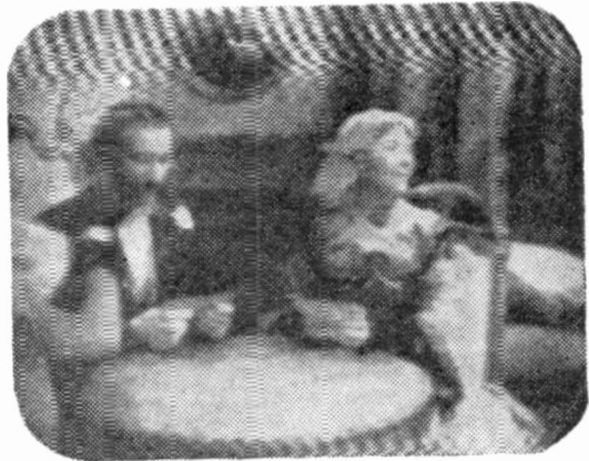
Effect of local interference—electro-medical apparatus
