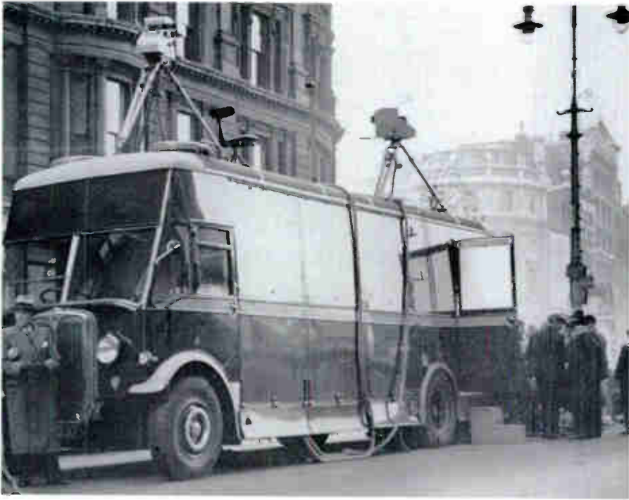
13f The Lord Mayor's Show, 9 November 1937. The Mobile Control van parked in Northumberland Avenue with two cameras positioned on the roof
