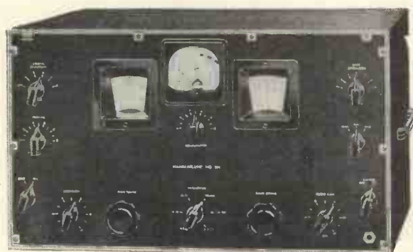
The very popular Hammarlund HQ-120X receiver, priced at £38.10s. It uses 12 valves and has a special crystal gate circuit.
