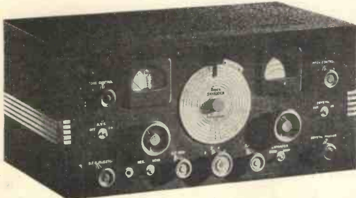
One of the most popular receivers in this country at the present time, despite competition, is still the Halli Craft SX17, which has two stages of R.F. and is priced at £39 10s., complete with crystal.
