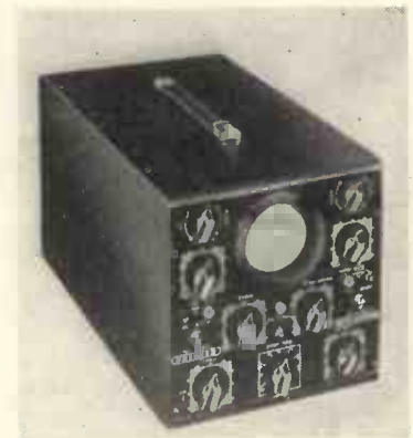
This oscilloscope by Premier Radio has a 3-in. tube and is priced at 10 gns.
