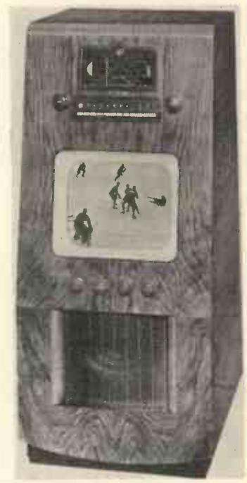
A console type receiver is the H.M.V. 1850. The picture size is 11½ in. by 9½ in., and in addition, an all-wave push-button radio is provided.
