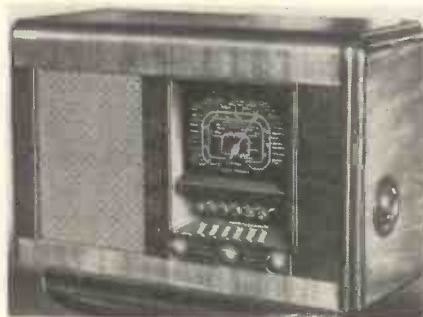
Cossor's five-valve model 81 all-wave superhet.
