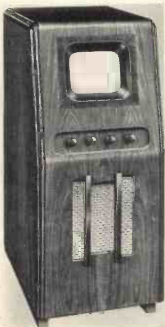
The Cossor 65 is a console model providing television sound and vision only. The picture measures 6 in. by 5 in.
