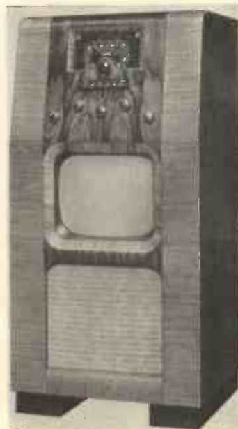
Another Decca receiver, but this model (the 46) includes an all-wave press-button radio in addition to television sound and vision.
