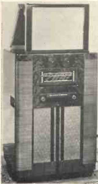
The Philips projection receiver giving a picture 18 in. by 14½ in.
