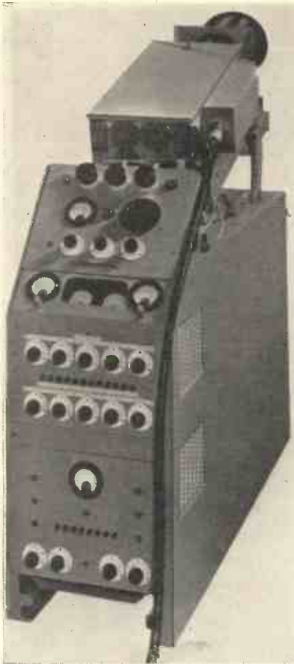
A rear view of the E.M.I. Projector showing the panels from which complete control of the equipment can be effected.
