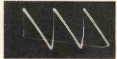
Fig. 14. Time base voltage with slow flyback stroke compared with Fig. 10.
