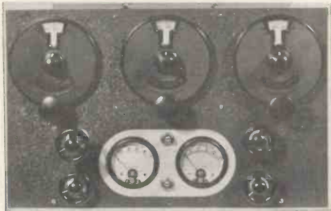
The panel lay-out gives a very commercial appearance while in practice there is only one tuning control after the band-spread condensers have been preset.
