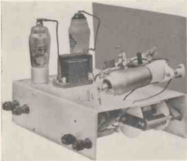
The tuning unit is fitted beneath the chassis so that the leads to the condenser and detector valve are kept short.
