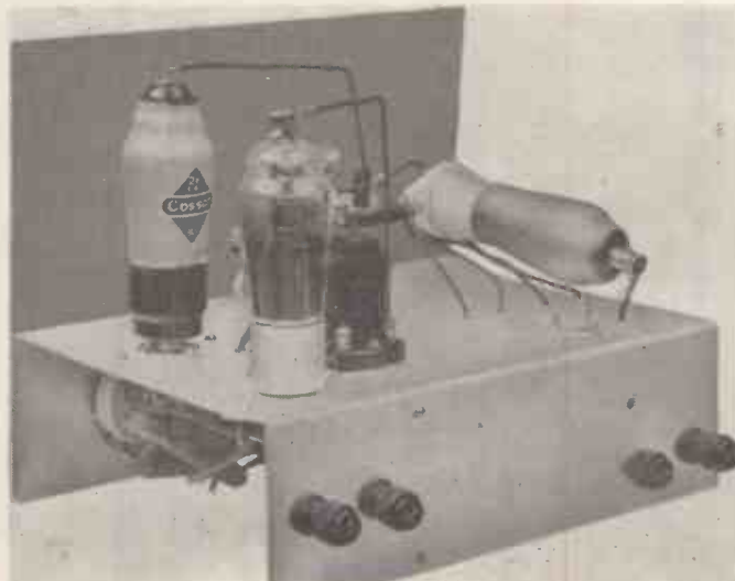
Most of the components are beneath the base-board while the aerial series condenser can be adjusted through the chassis.
