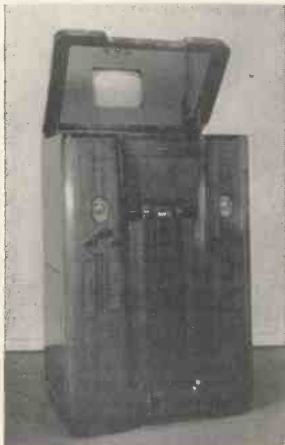
The Philco television receiver. The picture is observed in a mirror in the lid of the cabinet.
