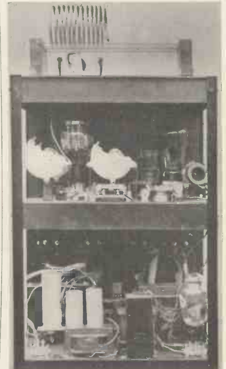
In the centre rack are the power packs one for the transmitter and the other for the speech amplifier.
