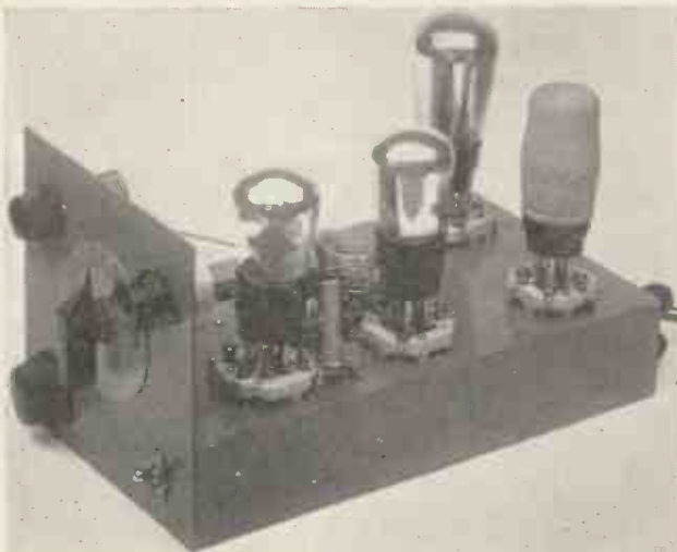
In the left-hand corner is the aerial series condenser. This is insulated from the panel. The remainder of the components on this panel are bolted on directly without bushing.
