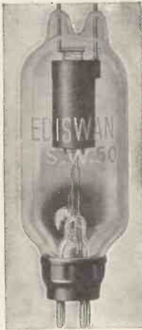
Fig. 1. This S.W. 501 has a graphite anode and a thoriated tungsten filament.
