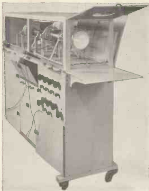
Fig. 6.—"Electron-Optica Bench" (G.E.C.) with vacuum pump for investigating cathode ray tube performance.
