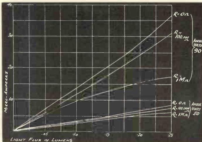
The effect of load resistance on the current-light curve at different anode voltages.
