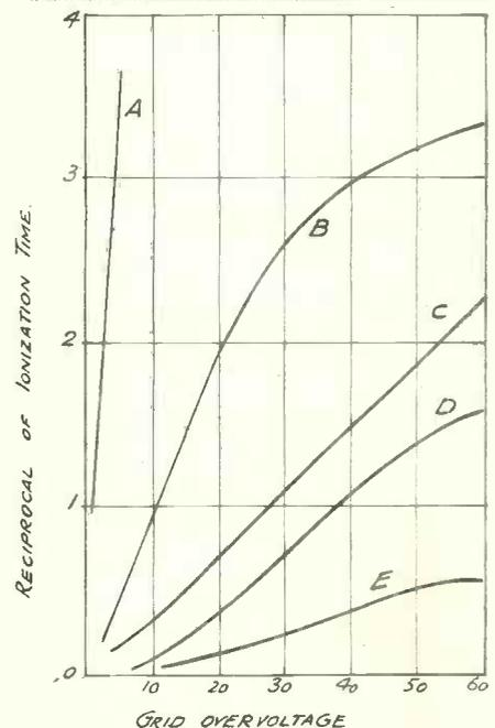
Fig. 3. Replotted curves showing the reciprocal of ionisation time as a function of grid overvoltage.
