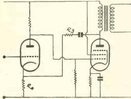
Fig. 3. Two methods of feeding back into a preceding stage. (3b corresponds to b of Fig. 2. and 3c to c of Fig. 2.)
