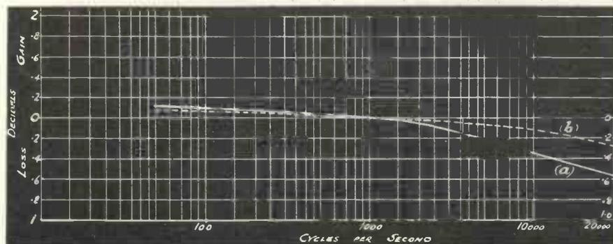
Frequency response curve of gas-filled photo electric cells. Cells measured with approximate gas factor of (a) .6 and (b) .25.
