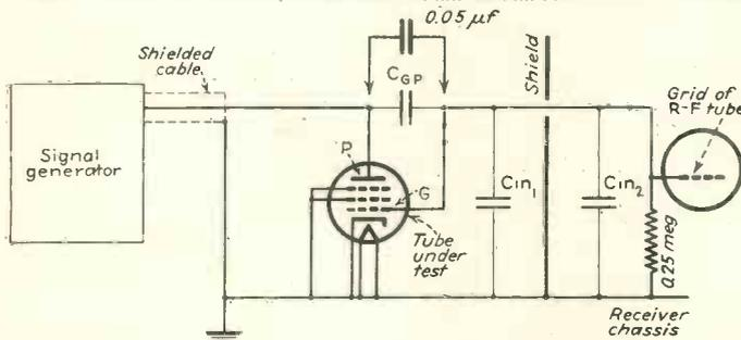
Circuit for determining valve capacity with a signal generator and radio receiver as measuring equipment.
