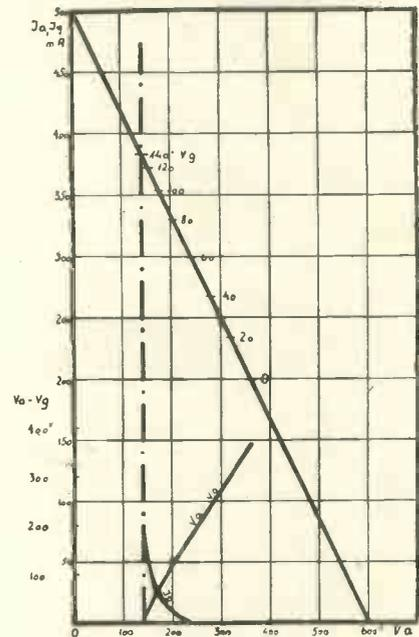
Fig. 11. Anode-voltage-grid and anode-current curve limits showing smallest permissible anode-load line of Tungram type P-25/450.
