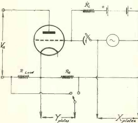
Fig. 13. Circuit for oscillographic observation of characteristics.
