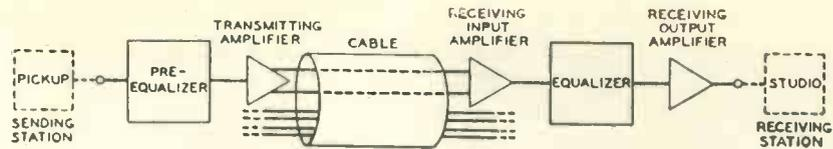
Fig. 2. Block diagram showing arrangement of equalisers.
