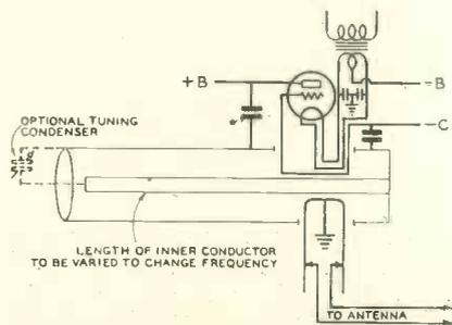
Single-tuned-circuit oscillator, cathode-above-earth type. The frequency can be varied either by the optional tuning condenser shown or by varying the length of the inner conductor of the concentric line.
