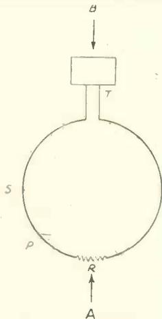
Fig. 1. Diagram showing principles of loop form of Beverage antenna.
