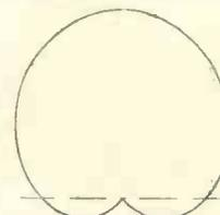
Fig. 4. Directional diagram of cardioid form.
