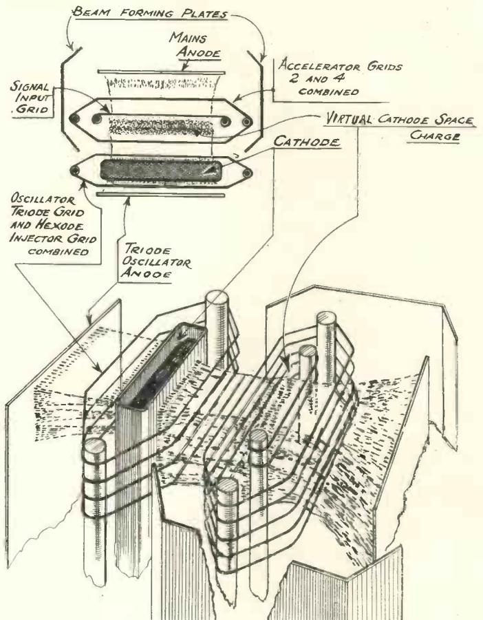
Though in America this valve is referred to as a triode hexode, a name it truly deserves, this may lead to some misunderstandings in this country as we refer to a valve as a triode hexode if the third grid of the hexode is internally connected to the triode grid.
