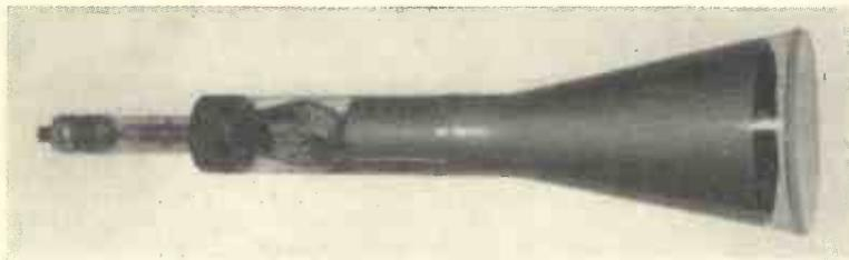
The B.T.H. cathode-ray tube with plane glass screen.
