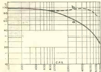
Fig. 1. Frequency response curves of type S5 cell in circuit. a—uncorrected. b—corrected.
