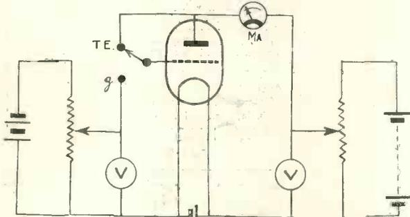
Fig. 2. Typical circuit for measuring static characteristics. The switch in the grid circuit enables measurements of total emission from the cathode to be obtained.
