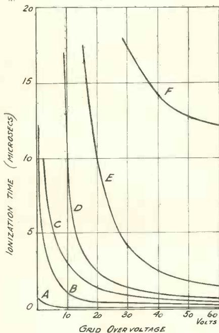
Fig. 2. Curves showing relationship between time of ionisation and grid overvoltage.
