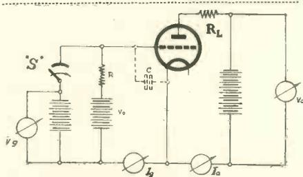
Fig. 9. Circuit including smallest permissible anode load.
