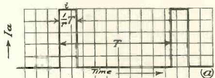
Fig. 3a. Ideal anode current waveform.
