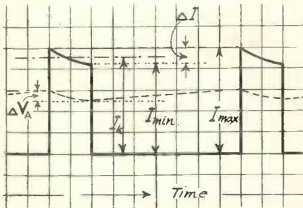
Fig. 14. Anode current waveform as a function of time.
