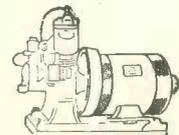
A 500-watt, single cyl. 2-stroke, water cooled, self-oiling Stuart Turner engine; mag. ign., coupled to 50/70 volts, 10 amps., shunt dynamo, 1,000 r.p.m. £16.
