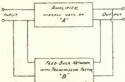
Fig. 1. Illustrating the principle of negative feedback.
