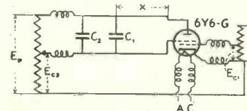
Schematic wiring diagram of the 6Y6-G ultra high frequency generator.
