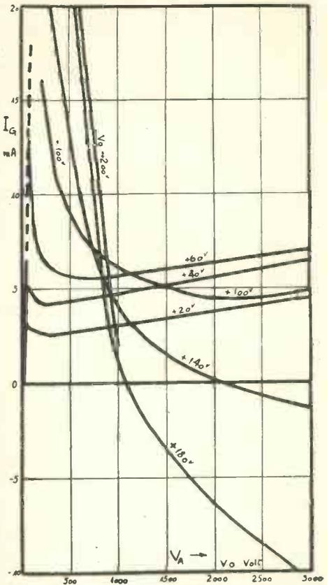
Fig. 7. Anode-volts-grid-current curves of the Tungram 0-300/3,000.
