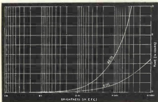
Fig. 1. Decay curves for AE(P) and F(P) type phosphors excited by standard source described in B.S./A.R.P./18, Dec., 1939.
