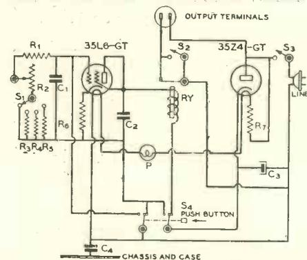
Wiring diagram of the printing timer.
