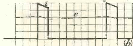
Fig. 3b. Approximate actual anode current (i) and voltage waveform (e).
