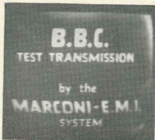
Right: Tube biased rather too brightly for photographing two tones black and white. The general curvature and angle of the Marconi-E.M.I. are due to two effects, one, curvature of tube, two local timing circuits not quite adjusted to incoming synchronising signal.
