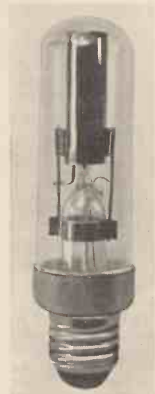
A crater lamp made for 120 line experiments
