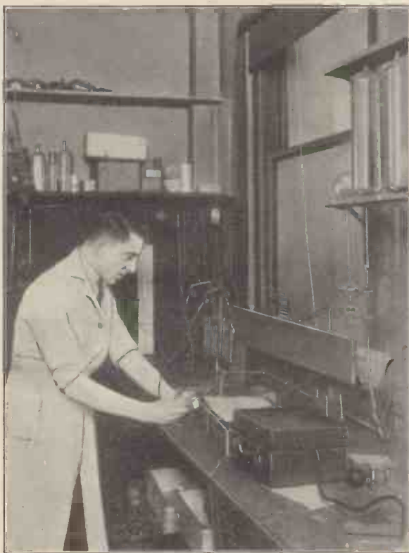
The interior of a neon tube filling laboratory. The pressure gauge can be seen on the left of the operator: on the bench is the lamp bank sealed to the pump
