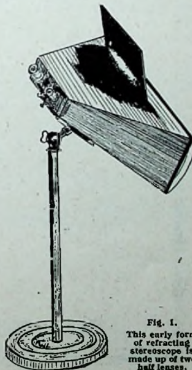
BREWSTER'S LENTICULAR STEREOSCOPE.
