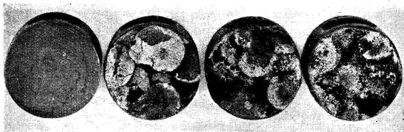
Fig. 7. Photomicrographs of copper-tungsten contacts after varying degrees of use. By courtesy of Mallory Metallurgical Products, Ltd.
