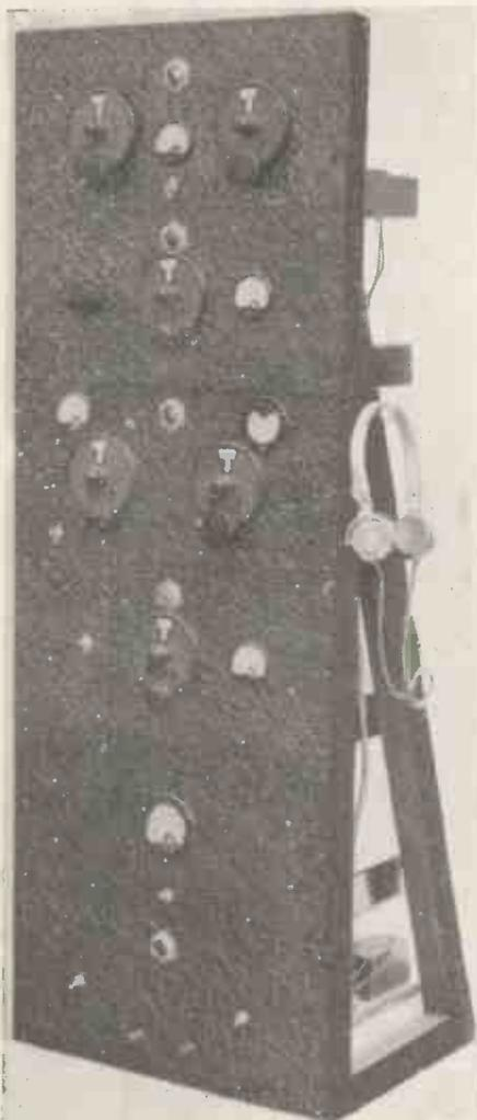
*The jack for the headphones in the speech monitor circuit is on the side of the top chassis. The second chassis from the bottom carries the bias supply with a switchable volt meter.*
