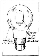
proof paper should now be cut out, slightly larger in size than the opening in the tin-foil, and this should be secured in place over the aperture by a little. glue applied at the top and bottom of the paper (A and B) only. If the glue is placed on all four edges it will be found difficult to make the paper lie over the bulb without creasing. Ordinary greaseproof paper of the type used for containing
