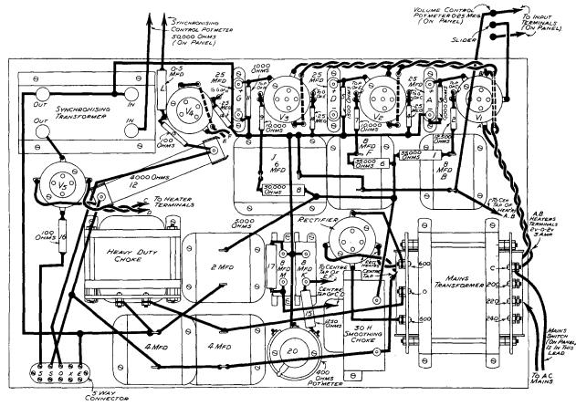
Fig. 3. The wiring diagram which is explained in detail in the text.
