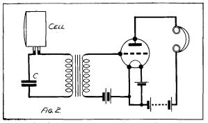
Connecting the cell to an L.F. amplifier through a condenser feed transformer.
