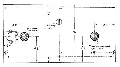
Diagram of the panel of the straight-line amplifier.
