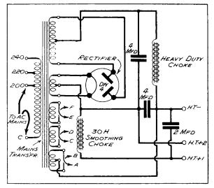
Fig. 2. Circuit of the H.T. eliminator.
