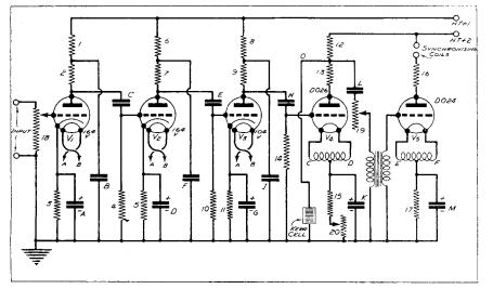
Fig. 1. Schematic circuit of the straight-line amplifier.
