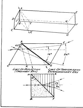
Fig. 1 (Top) Effect given by a natural crystal of Iceland Spar. Fig. 2 (Centre) Nicol's scheme for cutting the crystal. Fig. 3 (Below) Woollaston's prism.
