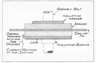
Fig. 3.—The Westinghouse dry metal rectifier unit is built up in sections on steel bolts such as the one illustrated above.
