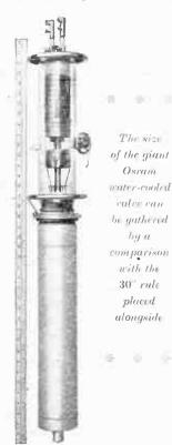
to the skill and ingenuity of British radio engineers and valve manufacturers. That it is a giant among valves is revealed by comparing a few of its dimensions with a standard wireless receiving valve, with which all owners of wireless sets are familiar :-Filament volts, 31.5 volts.
