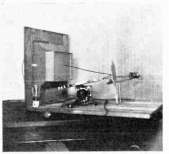
An interior view of Mr. Horst Hewel's home-made mirror drum vision apparatus. The ink line indica'es the path of the light heam.
