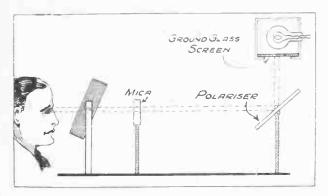
Fig. 3.—Details of a simple pelariser which is very inexpensive.
