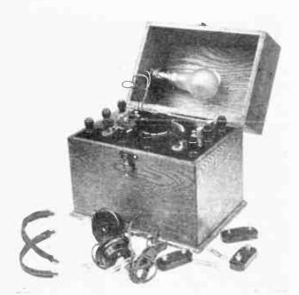
Not how the neon lump has been accommodated on the left-hand side of the lid. Be careful to ensure that the flexible leads do not y 1 jammed when the lid is closed.
