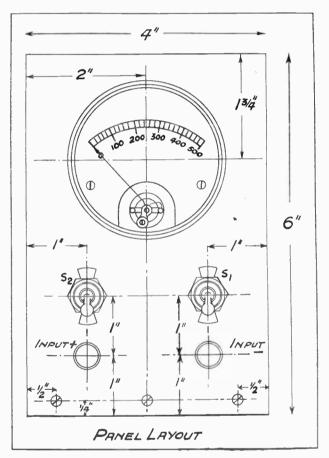
Fig. 2.—Complete details for marking out the panel prior to drilling operations.
