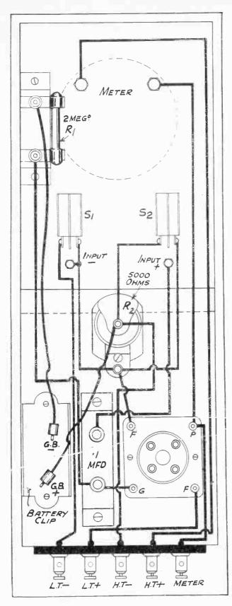
Fig. 3.—Neat and compact, little difficulty will be experienced in wiring if this diagram is followed carefully.
