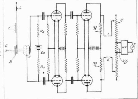
Fig. 1.— Diagram of the apparatus employed for the tests referred to in the text. L is a perforated disc, P a potentiometer. MV the amplifier and Tthe thermo voltmeter.
