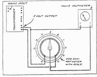
Fig. 4.—When calibrating the valve voltmeter access to an A.C. source is provided by a suitable step-down mains transformer.
