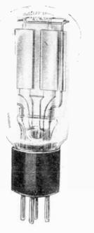
Modern types of full-wave thermionic valve rectifiers consist of a double plate and a single filament brought out to the four pins of a standard valve base. Here we see a Mullard D.W. 30 rectifier, which is most efficient.
