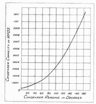
Fig. 2.—Plot out carefully the calibration curve for the variable condenser used in the Capacimeter.
