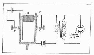
Fig. 1.—One method of obtaining a fixed number of pulses per second for feeding a neon lamp.
