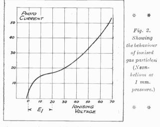
place over the mush level. There are limits to this possibility and in the first case care must be exercised that the voltage is not high enough to produce breakdown owing to the increasing slope of the curve.
