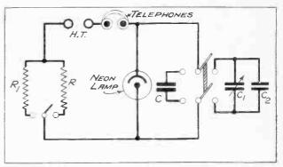
Fig. 3.—The the retical diagram for the t ster is shown here so that  $y \mid v$  can find exactly how the condens rs and resistance are referred to.
