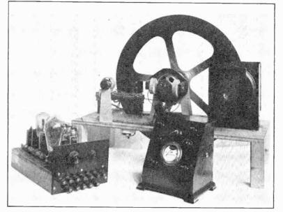
The unit ready for connecting between the vision amplifier and "Televisor" made up from a Baird set of parts.
