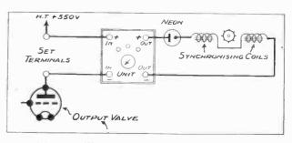
Fig. 5.--With a transformer output in the vision wireless receiver the unit is joined up in this manner.
