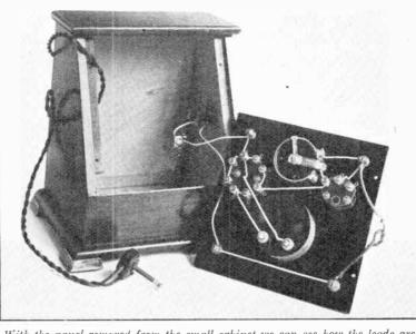
With the panel removed from the small cabinet we can see how the leads are joined to the jack.
