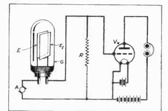
Fig. 3.—A cuprous oxide cell, Ruben's condenser type, together with the requisite electrical circuit.
