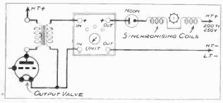
Fig. 6.—Showing how simple are the connections for a transformer and choke combination.
