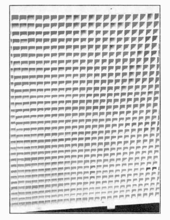
It has been mentioned on several occasions that the Baird lamp screen was made up in the form of a honeycomb. This illustration shows the framework used.
