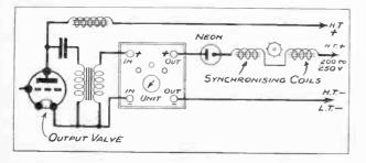
Fig. 4.—Linking the "output controller" to the vision apparatus when the output valve functions "directly."
