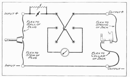
Fig. 2.—The theoretical diagram of the ``output controller,'' showing how the switches, jack, etc., are arranged.
