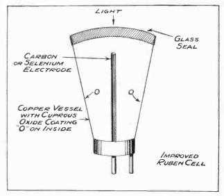
Fig. 4.—Illustrating an improved Ruben Cell.
