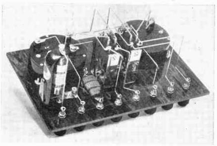
Notice how the wiring is carried out in neat. right-angled bends. Pay particular attention to the positioning of the telephone bobbins.
