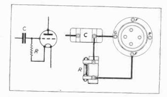
Fig. 1.—Urid leak rectification is shown both theoretically and pictorially in this diagram.
