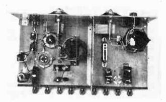
Here we see the high frequency and detector stages of a special unit designed for receiving the vision signals.
