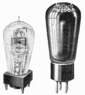
On the right, a super-power valve, while on the left is a valve designed to handle very large A.C. outputs.
