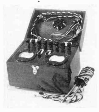
The complete "Teletester" in its compact box with the accessories mounted in the lid. The testing handles are shown at the sile.
