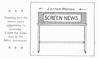
The interior of the apparatus contains an endless roll of varnished linen, which passes at intervals over rollers, and along which are regularly spaced small slots for the insertion of the letters. It is lined with thick felt to reduce the sound caused by the letters continually passing over the rollers. A general idea of the exterior of the apparatus is shown in the sketch.
