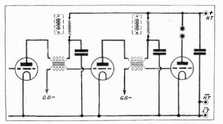
of each valve from the maximum tapping of the eliminator or battery through a separate resistance of such value that the requisite voltage drop is obtained. These resistances should be by-passed to earth by a fixed condenser of 2 mfds, capacity such as indicated in Fig. 2.
