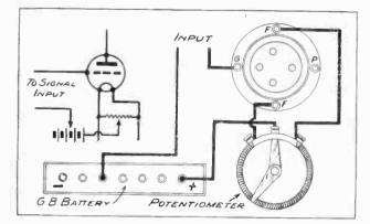
Fig. 2.—Notice the arrangements made for applying the correct grid bias in the case of an anode bend detector.
