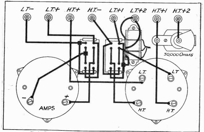
Fig. 2.—The wiring for the "Teletester" is perfectly straightforward and this diagram should be used in conjunction with the photographs.
