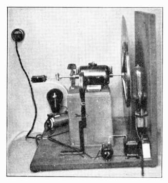
Josef Häring, of München, has successfully received the Baird television transmissions on the apparatus shown in the above photograph.
