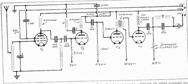
The circuit used by Mr Gordan E. Carden for the reception of the Baird transmissions. Although the values employed are not of the expensive kind, good results are claimed.
