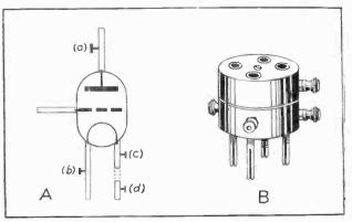
Fig. 3.—Theoretical and pictorial representations of the two pick-up adaptors which have been modified for the "Teletester."
