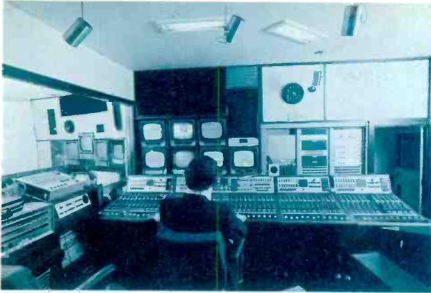
3. Sound is not the poor relation of television. This is the sound control suite of a modern studio where the levels from the many microphones are blended and balanced and effects added from audio tapes or discs.
