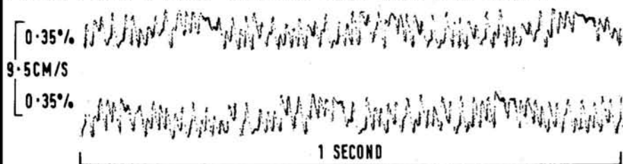
FIG. 1 PHILIPS 4307 RECORD-PLAY WOW AND FLUTTER
