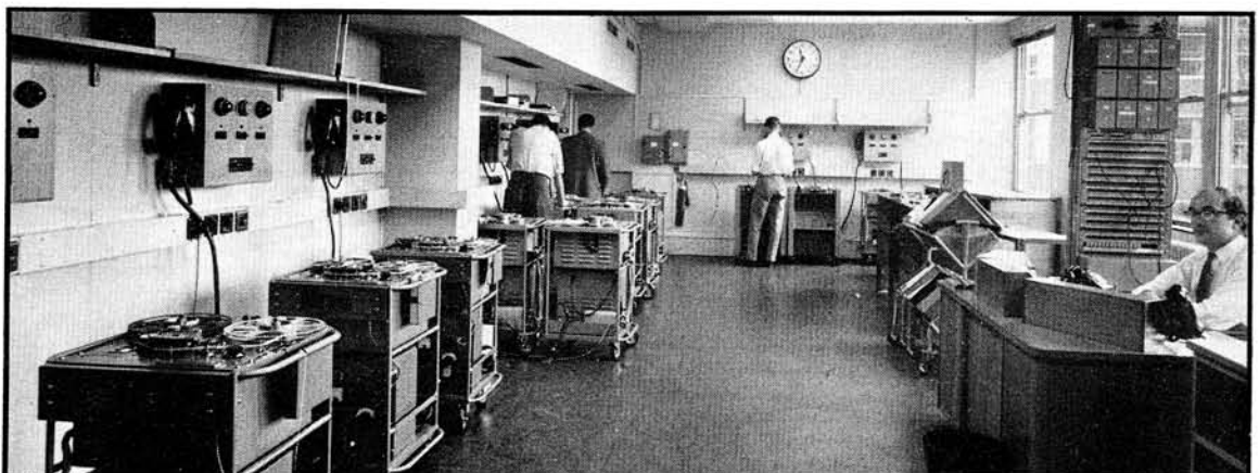
Trolley-mounted TR90 and (in distance) Leavers-Rich recorders at Central Recording Room H58, Broadcasting House Extension, 1962.
