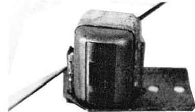
FIG. 7 Tin plate strap soldered to threaded brass.
