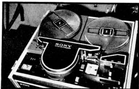
A Top deck of the Sony CV2100E, the dual-standard model with dubbing and editing facilities and AGC.
