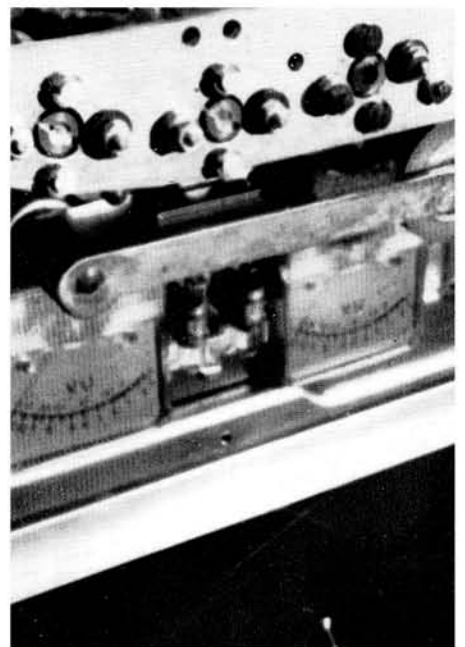
B View of the headplate showing alignment screws
