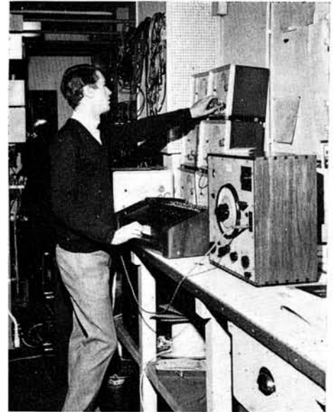
A corner of the BBC Radiophonics Workshop. The audio signal generators are coupled to a keyboard system providing varying degrees of attack and decay.
