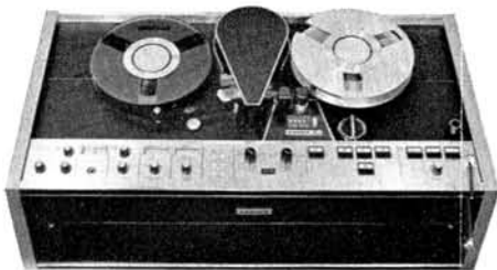
Ampex VR 7800 video recorder with built-in electronic editor
